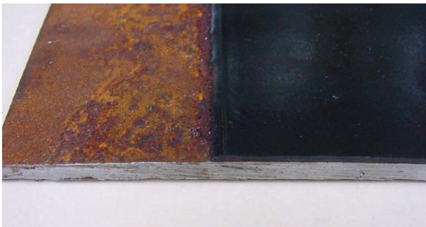
Figure 7. Corrosion stops right at the edge of the protective coating.
