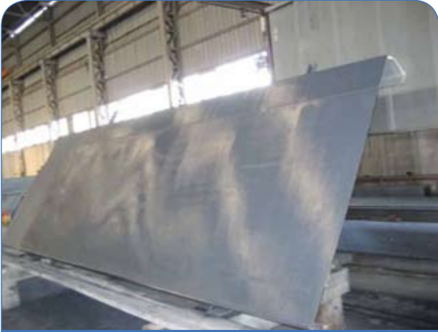
Figure 2. New filter plate coated with FlueGard-225SQC.
