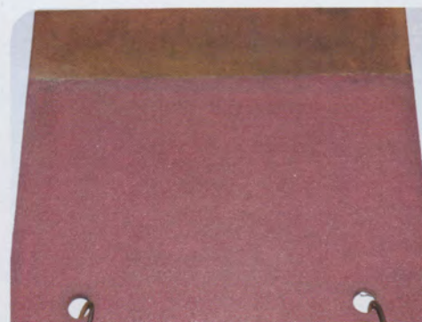
Figure 2. Test plate coated with ceramic FlueGard™-455CHT.
