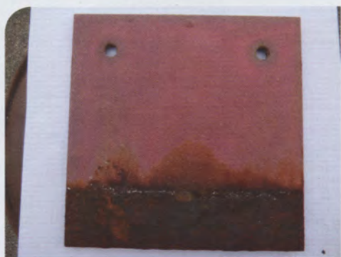
Figure 1. Exposed border corroded, no undercut damage.
